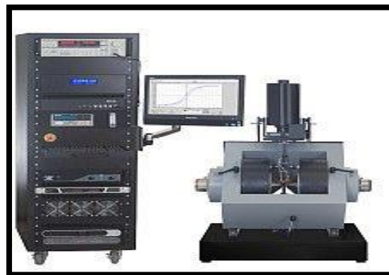
Figure (2.15): shows a simplified form of the VSM technology [95].
